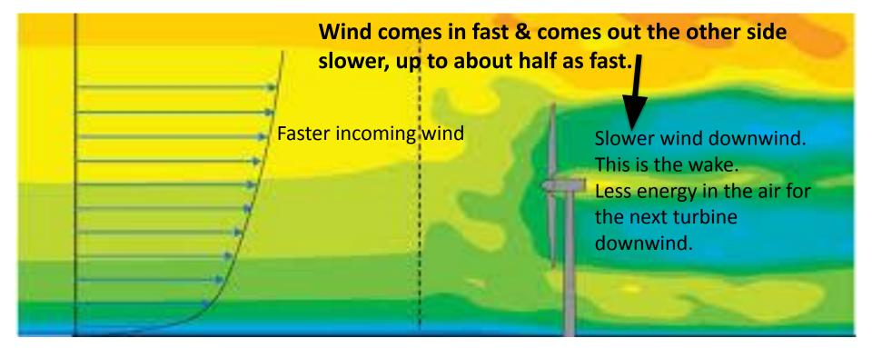
Based on the CEWEX field experiment (and others) no substantive impact on farming or environment due to wake wind speed changes. Wakes and their recovery rate are a critical wind farm design factor.
